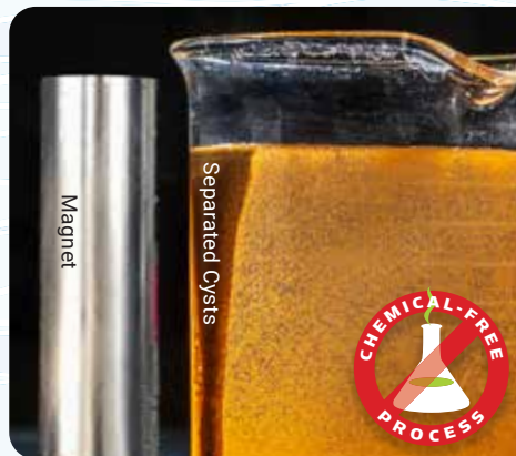
Demonstration of cysts magnetically drawn away from nauplii
